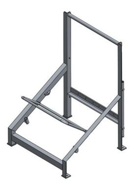
A rack designed to ensure that the liferaft will immediately drop into the water without assistance. For throw overboard liferafts weighting more than 185 kg sliding racks are mandatory, in accordance with the SOLAS convention chapter III regulation 16. Pre-drilled foundation holes have a diameter of Ø18.
