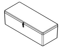
Material: Box, Fibre-reinforced plastic (GRP) Hinges, Stainless steel (SUS304) Handle, Stainless steel (SUS304)
