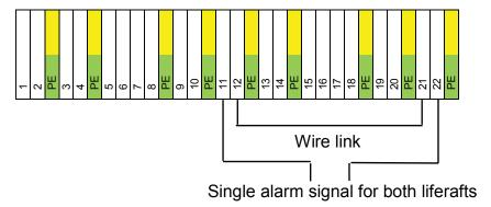
Example is for Thermal Control Box for three liferafts.
