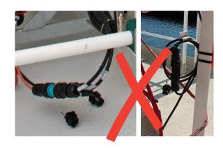
Use the protection cap when connectors is not assembled. Never let connector stay open when placed on open deck.
