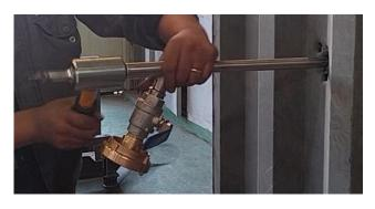
Hit the back part of lance using the hammer when lance needs to enter much deeper.
