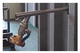
Open shut-off valve to shoot the water to the container inside.
