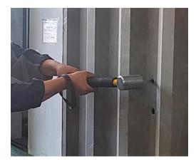
Punch on container wall by special hammer.
