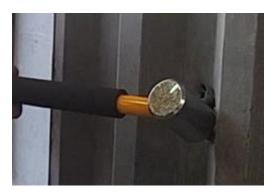
Move up and down or zigzag to make a hole bigger with a hammer.
