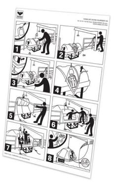
Launching instruction for 12DKF+, 16DKF+, 20DKF+, 25DKF+ and 35DKF+ in round container (SOLAS A and B) and 25DKFS and 39DKFS in round container (SOLAS A and B) in cradle.
