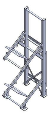
A rack designed to ensure that the liferaft will immediately drop into the water without assistance. For throw overboard liferafts weighting more than 185 kg sliding ramps are mandatory, in accordance with the SOLAS convention chapter III regulation 16. The rack should be mounted by welding to the hull foundation support.
