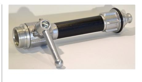
The CMM branchpipes are available in sizes 2" and 2½". In order to protect the branchpipe operator against heat and smoke, it can set up a water curtain, in addition to the jet and spray water screen. The exit angle can be continuously changed from 0° to 160°.
