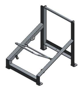
A sliding rack designed to ensure that the liferaft will immediately drop into the water without assistance. For throw overboard liferafts weighting more than 185 kg sliding ramps are mandatory, in accordance with the SOLAS convention chapter III regulation 16. Pre-drilled foundation holes have a diameter of Ø18.
