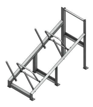
A rack designed to ensure that the liferaft will immediately drop into the water without assistance. For throw overboard liferafts weighting more than 185 kg sliding ramps are mandatory, in accordance with the SOLAS convention chapter III regulation 16. Pre-drilled foundation holes have a diameter of Ø18.
