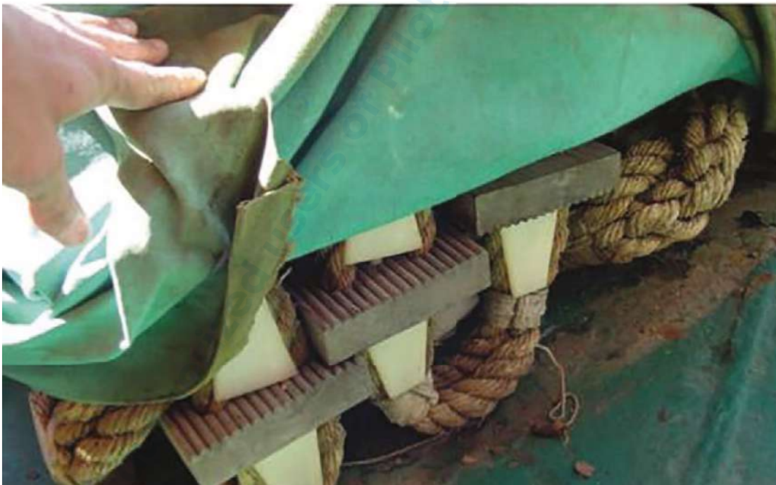
Figure B.2 — Embarkation ladder resting on deck, exposed to attack by water and cleaning chemicals
