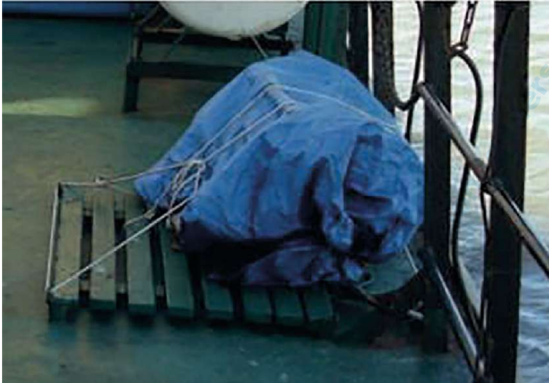
Figure B.3 — Embarkation ladder stowed clear of the deck and suitably covered
