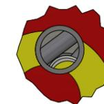
Hook is open or in automatic release mode position (Hook is not locked)
