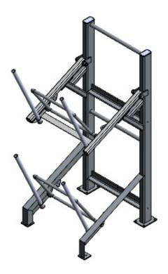
A column rack designed to ensure that the liferafts will immediately drop into the water without assistance. For throw overboard liferafts weighting more than 185 kg sliding ramps are mandatory, in accordance with the SOLAS convention chapter III regulation 16. Pre-drilled foundation holes have a diameter of Ø14.
