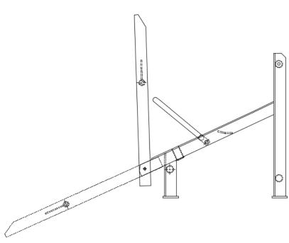
A rack designed to ensure that the liferaft will immediately drop into the water without assistance. For throw overboard liferafts weighting more than 185 kg sliding ramps are mandatory, in accordance with the SOLAS convention chapter III regulation 16. Pre-drilled foundation holes have a diameter of Ø17.
