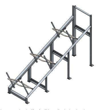
A sliding rack designed to ensure that the liferaft will immediately drop into the water without assistance. For throw overboard liferafts weighting more than 185 kg sliding ramps are mandatory, in accordance with the SOLAS convention chapter III regulation 16. Pre-drilled foundation holes have a diameter of  $\emptyset$ 18.
