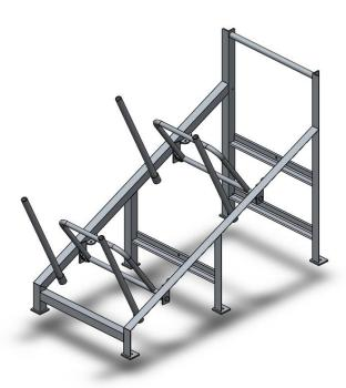
A rack designed to ensure that the liferaft will immediately drop into the water without assistance. Sliding ramps are mandatory for throw overboard liferafts weighting more than 185 kg in accordance with the SOLAS convention chapter III regulation 16. Pre-drilled foundation holes have a diameter of Ø14.
