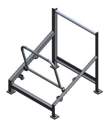
A rack designed to ensure that the liferaft will immediately drop into the water without assistance. For throw overboard liferafts weighting more than 185 kg sliding ramps are mandatory, in accordance with the SOLAS convention chapter III regulation 16. Pre-drilled foundation holes have a diameter of Ø14.
