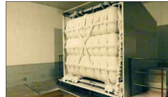
VIKING VEC Plus™ Polar system ice tested at -30°C
