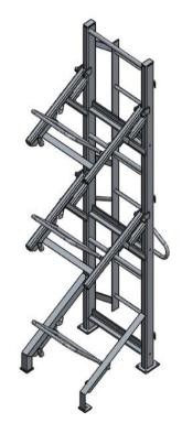
A column rack designed to ensure that the liferafts will immediately drop into the water without assistance. For throw overboard liferafts weighting more than 185 kg sliding ramps are mandatory, in accordance with the SOLAS convention chapter III regulation 16. Pre-drilled foundation holes have a diameter of Ø14.
