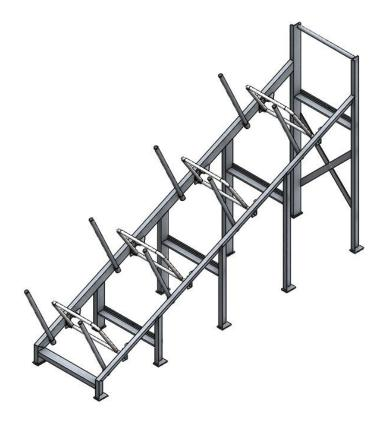
A rack designed to ensure that the liferaft will immediately drop into the water without assistance. For throw overboard liferafts weighting more than 185 kg sliding ramps are mandatory, in accordance with the SOLAS convention chapter III regulation 16. The rack should be mounted by welding to the hull.
