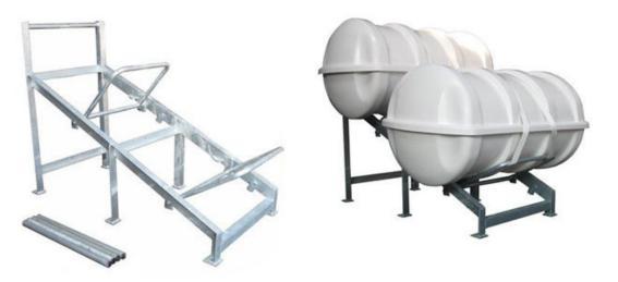
A sliding rack designed to ensure that the liferaft will immediately drop into the water without assistance. For throw overboard liferafts weighting more than 185 kg sliding ramps are mandatory, in accordance with the SOLAS convention chapter III regulation 16. Pre-drilled foundation holes have a diameter of Ø14.
